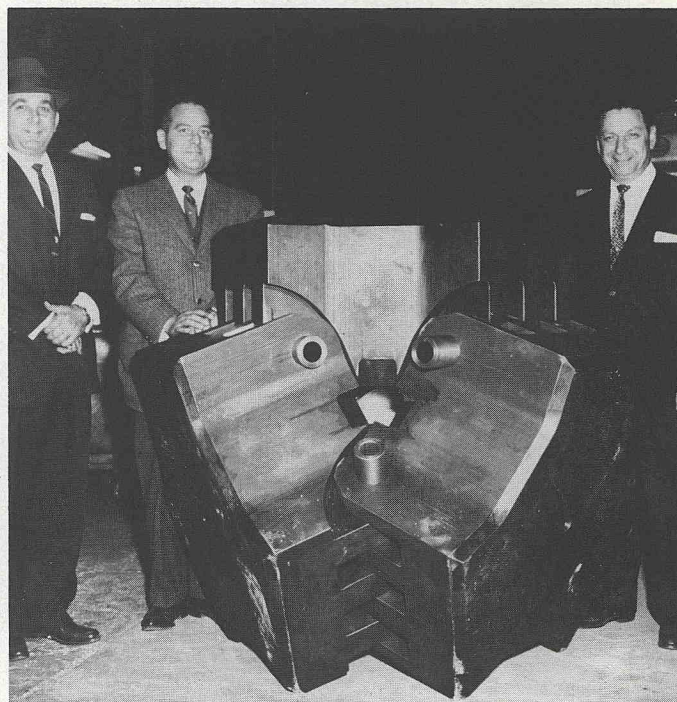
Fig. 19 Assembly of a 2000/8000 ton tetrahedral hinge unit
